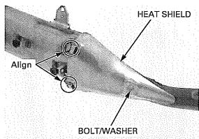
Install a new gasket onto the exhaust pipe. Install the muffler to the exhaust pipe.
