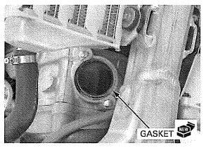
Install the exhaust pipe and tighten the nuts to the specified torque.
