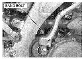
Remove the muffler mounting bolts, washer and muffler.
