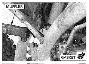
Install the washer and muffler mounting bolts. Tighten the muffler joint band bolt to the specified torque.
