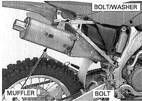
Remove the bolt, washer and heat shield from the muffler.
