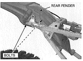
Remove the sub-frame upper mounting bolts and sub-frame.
