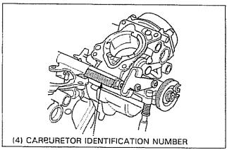
(4) The carburetor indentification number is stamped on the carburetor body intake side.
