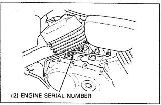
(2) The engine serial number is stamped on the right side of the upper crankcsase.
