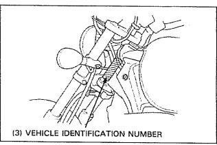
(3) The vehicle Identification Number (VIN) is located on the Safety Certification Label on the left side of the steering head.
