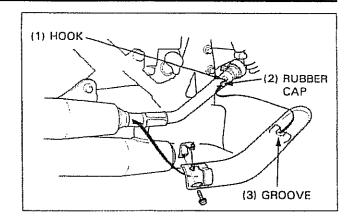
Adjust the clearance by moving the protector.
